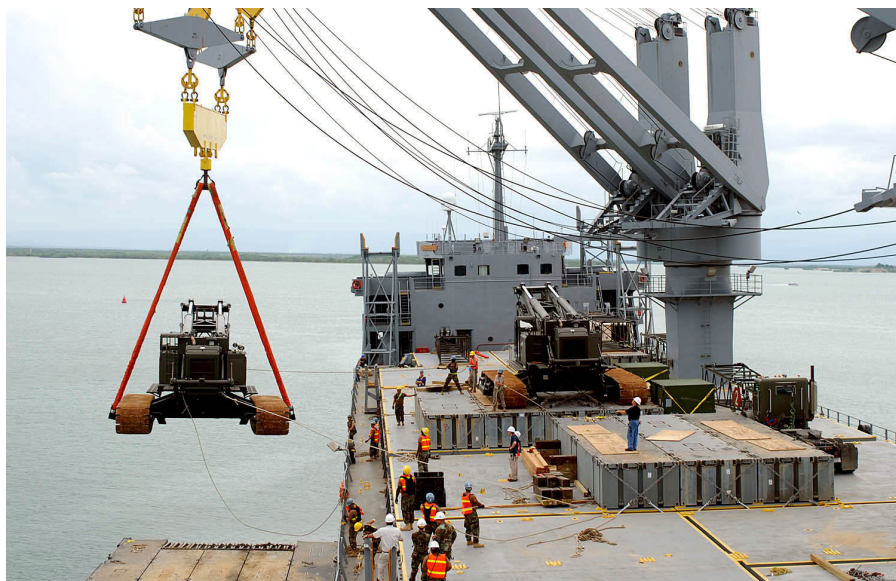
MacGregor's APC system uses motion data to make cargo landing and lifting operations as smooth and safe as possible
