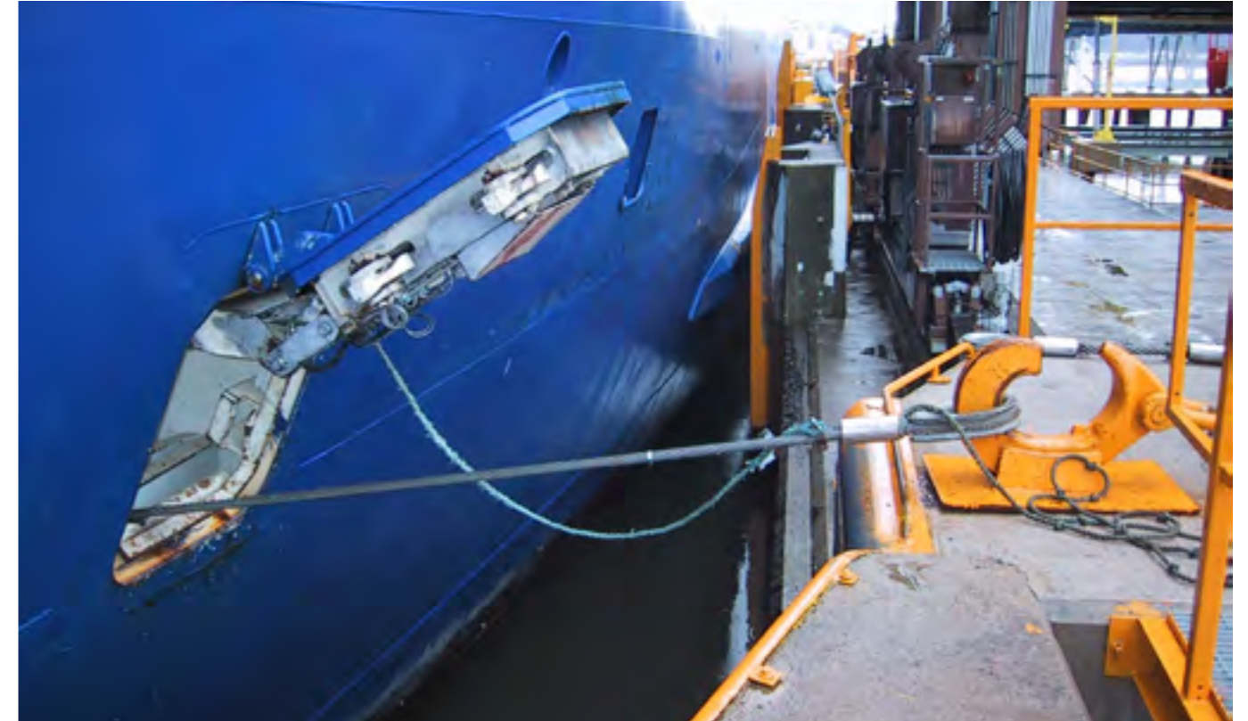
MOOREX® on board equipped with a weathertight side shell door, which can be opened inwards or outwards.
