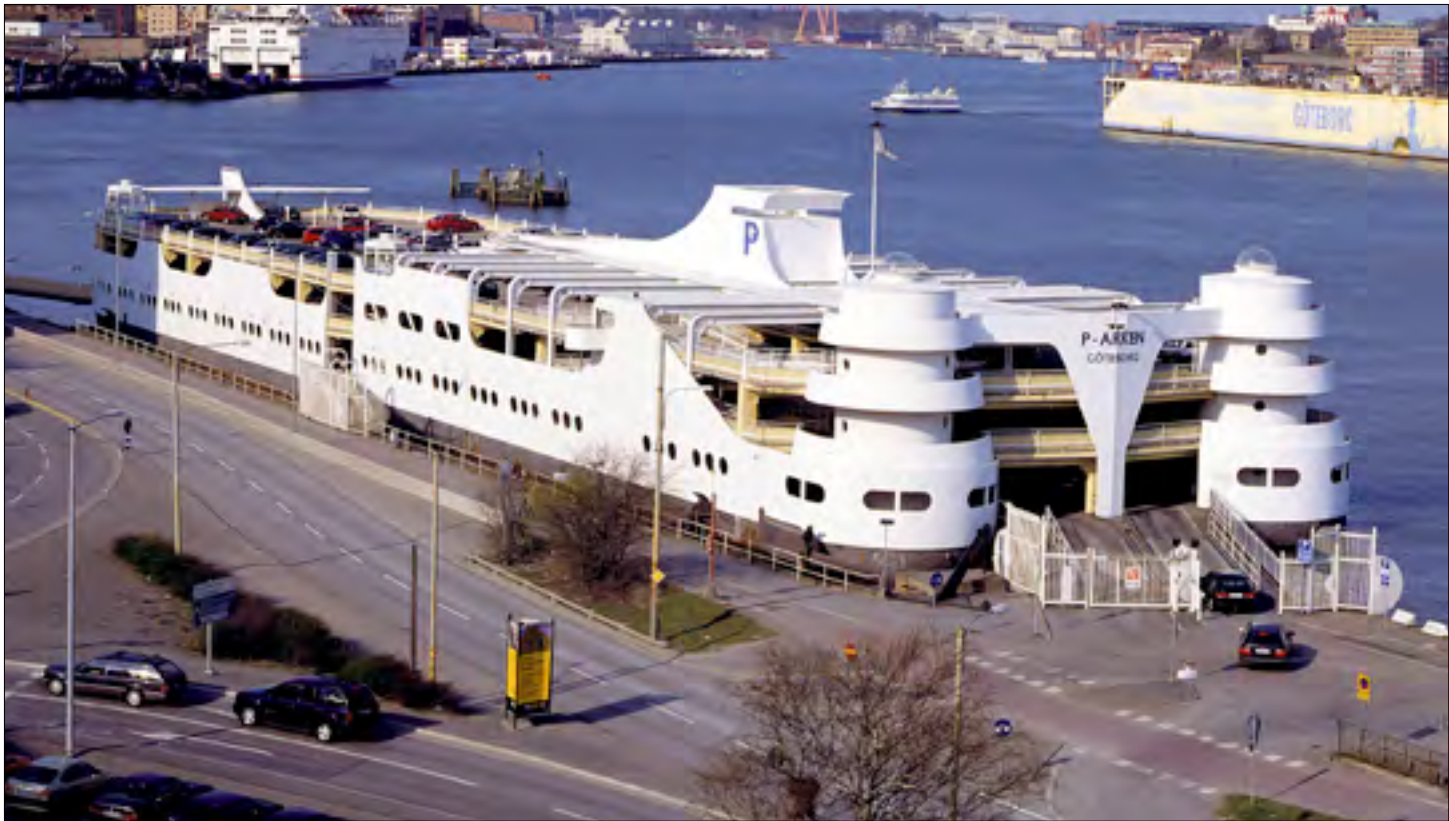
More than 400 cars can park in the P-Ark, the floating car park garage in Gothenburg, Sweden, 1991
